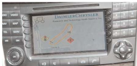
Pictured above is the view of the screen inside of the console of the Mercedes Benz Test Car, which gave the driver their location in the construction zone. The car would also speak to the driver and let them know that they were entering a construction zone, so the driver could adjust to the speed.
