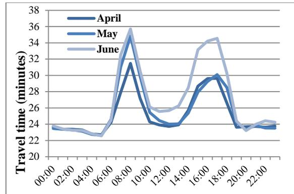
**Figure 4: Travel time comparisons, I-495 from I-66 to I-95 segment Counterclockwise, April, May, June, 2012.**
