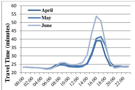
**Figure 3: Travel time comparisons, I-495 from I-66 to I-95 segment Clockwise, April, May, June, 2012.**
