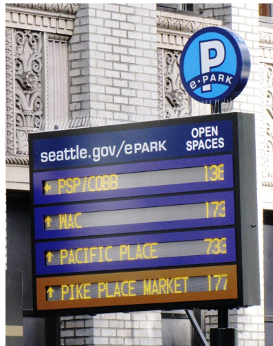
Figure 13. Photo. An e-Park dynamic message sign shows the number of open parking spaces at nearby parking facilities.
