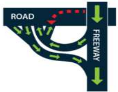
Side-by-side (partial cloverleaf) highway entrances and exit ramps
